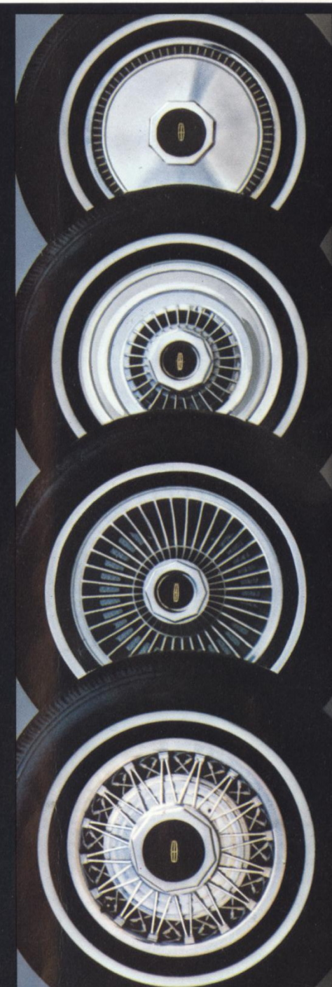
Top to bottom: standard luxury wheel cover and these options: forged aluminum wheel, turbine-style cast aluminum wheel and wire wheel cover.
